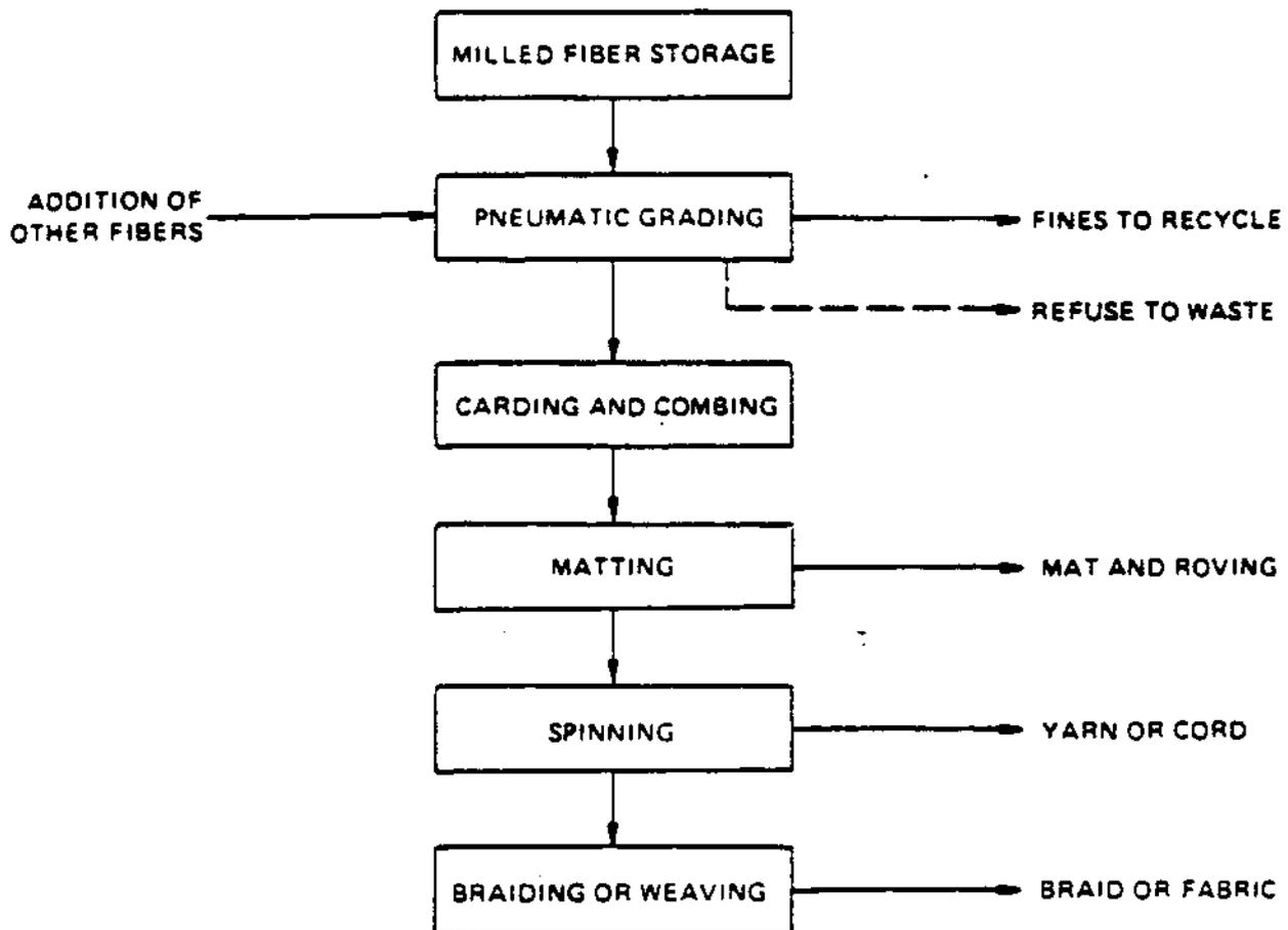
Figure 1. Manufacturing steps for asbestos textiles.
