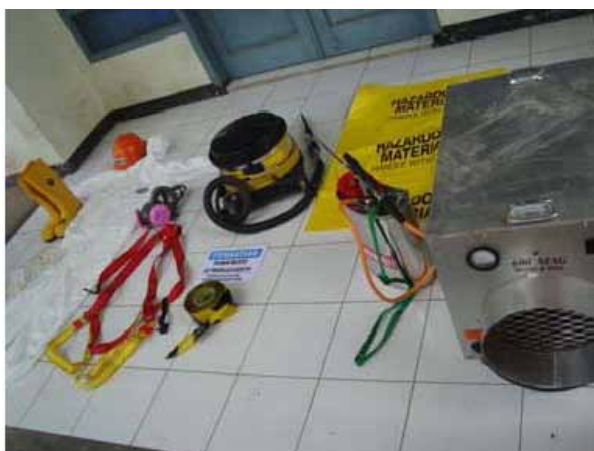
Picture 3. Equipment Used for the Asbestos Removal Project
